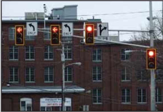
Exhibit 3: Signals with retroreflective backplates in the City of Nashua, New Hampshire. (Source: VHB)
