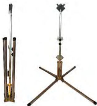
SS548AE Full-size stand with two stage dual spring action base with extended mast enabling a 21" & 5 ft. mounting height; kick release aluminum legs. Supports roll-up and rigid signs.
