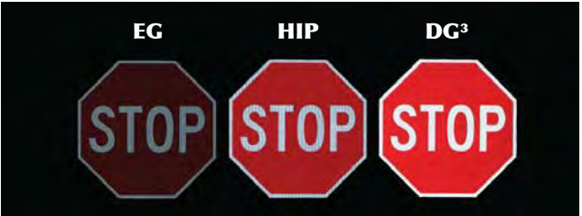
Nighttime comparison of Engineer Grade (Type I), High Intensity Prismatic (Type III/IV) and DG3 (Type XI) Reflective Sheeting.
